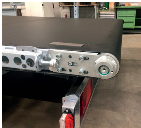
Electrically operated conveyor belt with gear transmission
