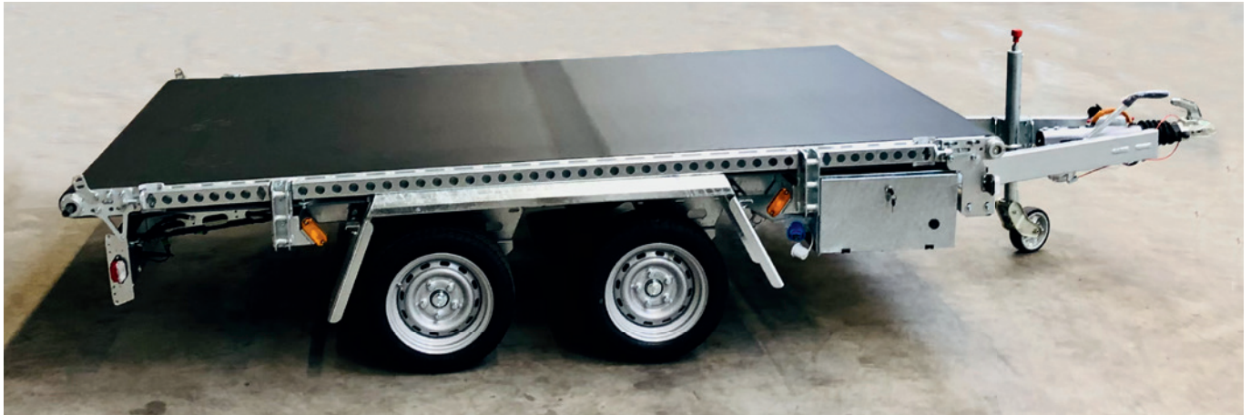
Electrically operated conveyor belt with gear transmission
